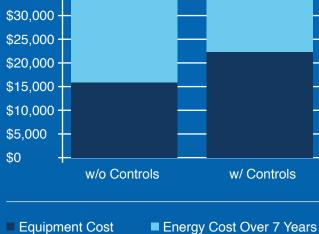
This example shows the cost savings for 200 LED luminaires at 34W each with an electricity rate of \$0.20/kWh and 3,132 annual hours of operation. Assuming an average of 63% control factor savings.
