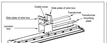
Install the mounting plate and transformer on the back of driver box with screws as shown.
