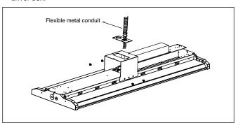
4. Connect the end of the conduit to the outlet box. Install the side plate and access plate with screws.
