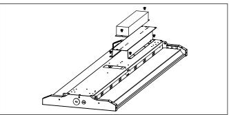
Make wiring connection and affix the junction box to the side of driver box.
