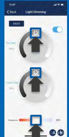
The dimming page varies according to the type of the lights, from left to right are dimming pages for mono-dimmable, tunable white, RGB dimmable and direct/in-direct dimmable light. Please click and slide the controls to dim the lights.
