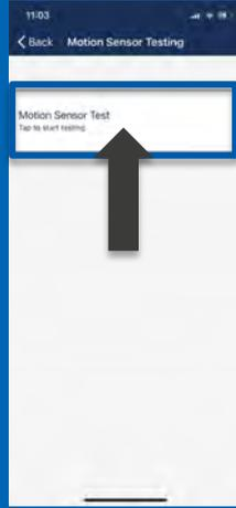
Click "Motion sensor test" and all lights with motion sensors will be turned off but motion sensors are working. Movement inside the motion sensor detection area will trigger and turn on the lights.
