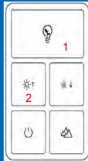
Press the button 1 and 2 together and hold for 2 seconds and then release.
