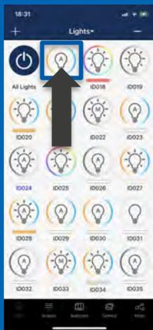
Please make sure the lights are in auto mode before you set it manually. The light is in auto mode when there is an "A" in the light bulb icon. You may set the light to auto mode by turning on the light or clicking the "Auto" button on a group.
