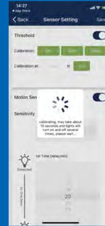
It will prompt a notice message during the calibration process. Please wait until the calibration ends. The light will quick flash several times if it failed to calculate the OFF threshold successfully. Please try to calibrate it another time. One possible reason for calibration failure is because there is too much ambient light so do not calibrate it during broad day light.
