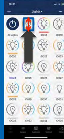
Sliding up and down on a tunable white light's icon can quickly change its color temperature.
