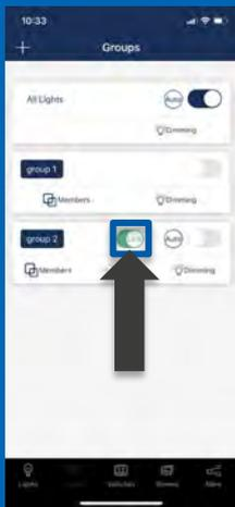
Click the "Link" toggle button for a group to turn the linkage function on/off.
