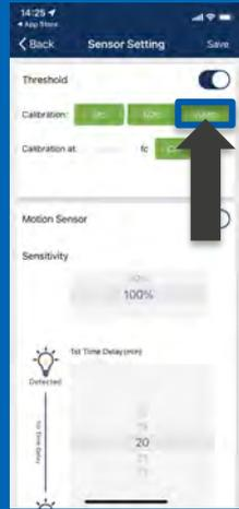
For photocell sensors, the default ON/OFF threshold is 10/60 fc. User may change the thresholds. Clicking the button of 5fc/ 50fc/100fc will set 5/50/100 fc as ON threshold respectively and the lights will turn on/off several times to auto-calculate the OFF threshold. User may input a specified fc value as ON threshold and click the “Cal” button to calculate the OFF threshold based on it.
