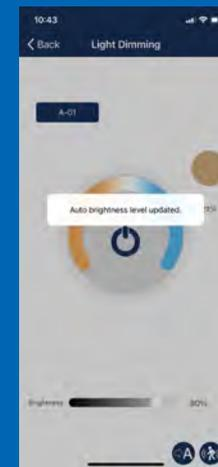
The lights will read the current light level from sensors and also record the current color temperature and save them as the auto light level.
