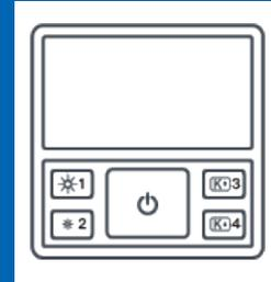
Press the button 1 and 3 together and hold for 2 seconds and then release.
