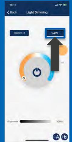
Please note that the wattage is the rated wattage after top-trim settings. E.g., you should input 24 for a 30 watt light with 80% of top-trim setting.
