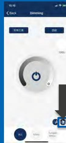
If there are lights with sensors in this group, then you may set the sensors parameter by clicking the sensor icon on the bottom right corner.
