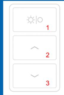
Press the button 1 and 3 together and hold for 2 seconds and then release.
