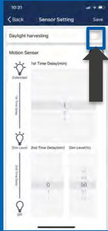
You may enable/disable sensors and set the parameters for the PIR sensor. Please click the "Save" button on the top right corner to save the settings. (Enable, disable sensors will become effect immediately without saving.)
