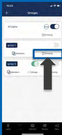
Click the "Dimming" button on the bottom right corner of a group to dim the lights in this group.
