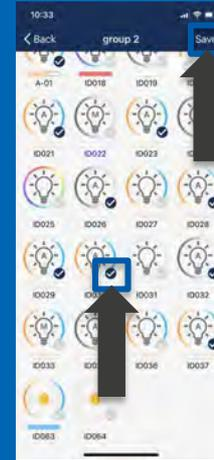
Click the checkbox on the bottom right corner of a light's icon to select/deselect the light. Click the "Save" button in the top right corner after selecting all appropriate members to save the group.
