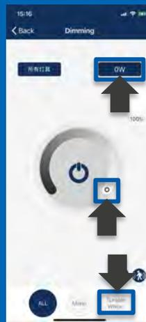
The available dimming control in the dimming page is shown according to the light type in this group. The light types in the group are shown on the bottom of the dimming page. You may choose to dim certain types of lights in this group. You may also set the wattage for all lights in this group in a batch. This is not the total wattage of the group, it is the wattage for each light in this group.
