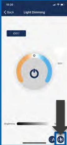
There is a sensor setting icon on the bottom right corner of the dimming page, click this icon to set the sensor's parameters.
