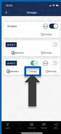
Click the "Linkage" button of a group to set the linkage brightness level of this group.
