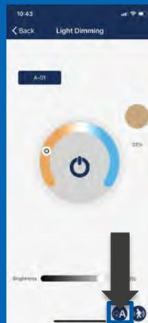
Use the app to dim the light or group when it is in auto mode to confirm the light level and color temperature are appropriate for auto lighting. Then click the "Set auto light level" button at the bottom.
