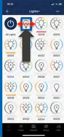
Sliding left and right on a light's icon can quickly dim the light up and down.
